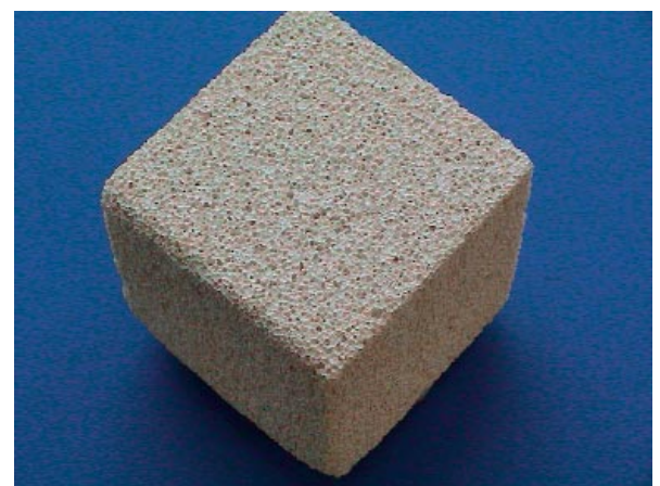
Fig. 6 Inorganic foam bonded with monoaluminium phosphate
